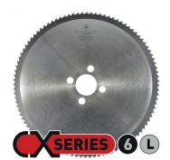
The PVD coated CX 6-L saw blade has specifically been designed for cutting austenitic stainless steel bars with a diameter larger than 35mm at very high production rates. With its dedicated geometry, very fast cutting and good surface finish can be achieved.
