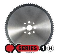
Applying a new saw body design, new tooth geometries and a new type of PVD coating, the CX 1-H saw blade has specifically been designed for cutting high tensile carbon steel (>  $900 \text{ N/mm}^2$ , carbon content  $\geq 0.60\%$ ) at very high production rates. It is also very suitable for cutting ferritic, martensitic and duplex stainless steel bars with a diameter larger than 35 mm.
