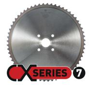
CX 7 is a Cermet tipped, PVD coated saw blade dedicated to cutting carbon steel (carbon content < 0.60%) with a low to medium tensile strength up to 750 N/mm². The best blade performance is being achieved when cutting lower tensile materials. On many applications, a blade life of 50 m² and more can be achieved.
