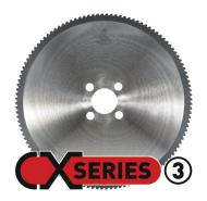
The CX3saw blade has been developed for cutting tubes on high performance automatic sawing machines, at a higher maximum cutting speed than possible with HSS saw blades. It is most effective on sawing machines with accurate control of chip load and variable feed rate. Bigger tips are applied at pitches > 9mm for added stability.
